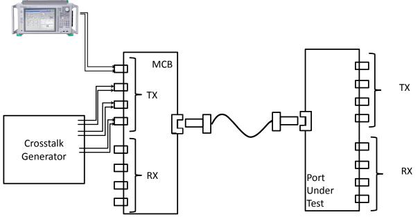
Figure 2. Test setup for FDR RX tolerance testing with linear cables.
