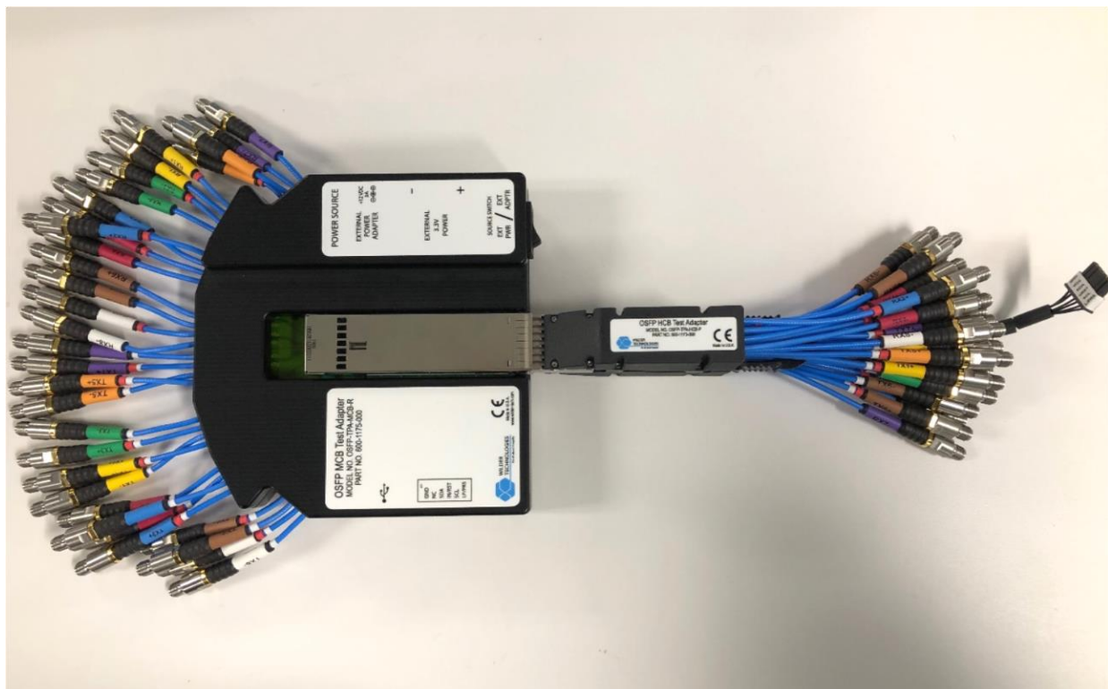
Wilder OSFP mated Module Compliance Board (MCB) and Host Compliance Board (HCB)
